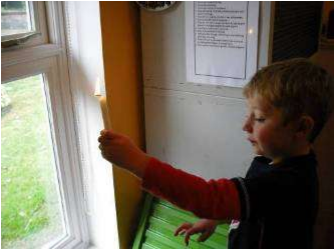
Children doing the environmental audit and checking for draughts with a candle
